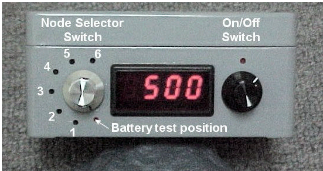
Figure 3. Handheld readout unit - front view, showing switches, battery test position, and node reading position.
