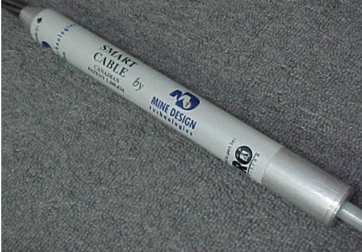
Figure 1. Electronic readout head for SMART instruments. Small diameter (33 mm) designed to fit inside the collar of 50 mm borehole.
