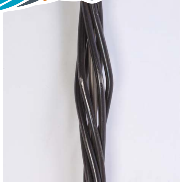
SMART cables are indistinguishable from regular cable bolts in the bond section.
